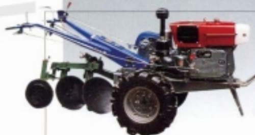
FITTED WITH DISK PLOUGH MODEL 1LY-220
