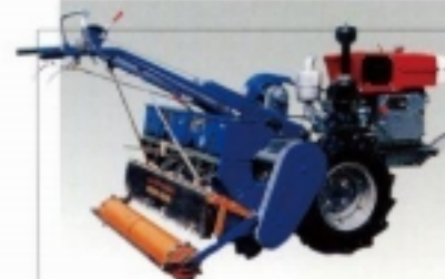
FITTED WITH CULTIVATOR DRILL MODEL 2BG-6A
