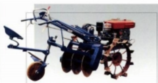
FITTED WITH POWER DRIVEN DISK PLOUGH MODEL 1LYQ-300
